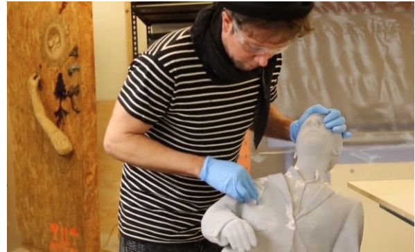
Figure 5. Video still of Louis Pratt sanding an FDM print prior to moulding and casting in wax. The wax pattern is then casting in metal. Image sourced from Louis Pratt, "About", accessed 17 September, 2020, https://www.louispratt.com/about .
