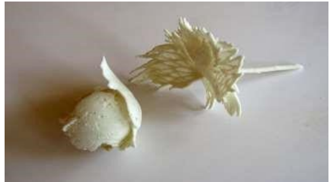
Figure 9. The design was FDM printed using polylactic acid using a Flashforge Adventurer 3.
