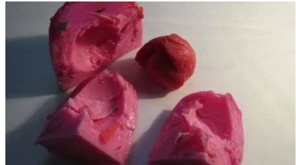
Figures 11 - 12. After SLA printing a version using photo-polymer tough resin, the object was moulded in silicone and cast in wax. The loss in detail was significant.
