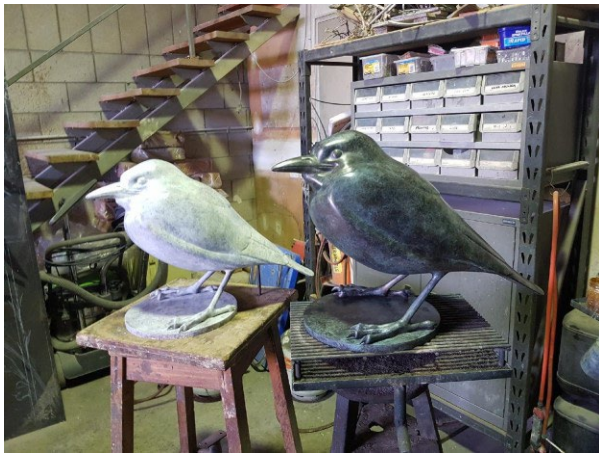
Figure 7. Image supplied by Perides Art Foundry of a 3d printed pattern and a cast bronze sculpture.
