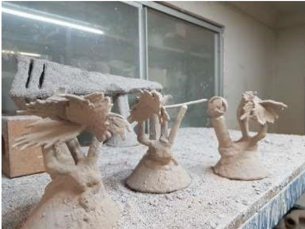
Figure 8. An image supplied by Perides Art Foundry of the ceramic moulds resulting from investment casting.
