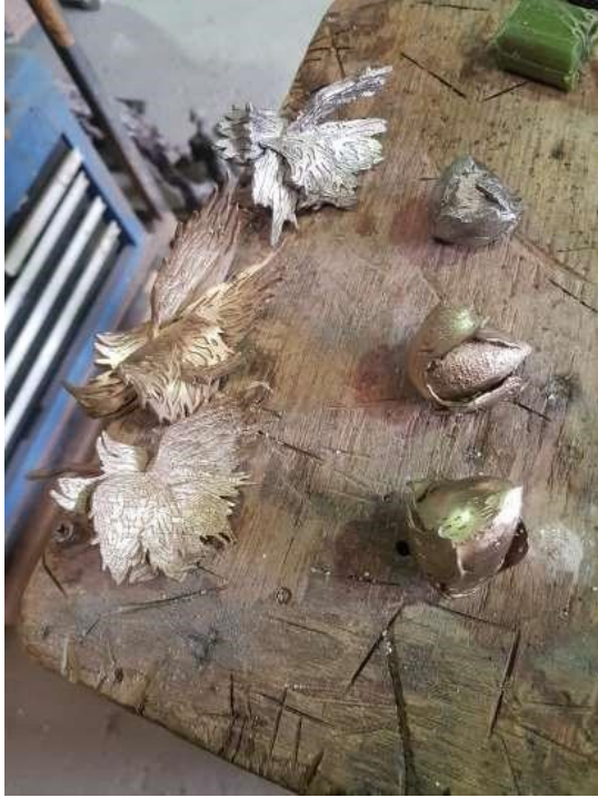
Figure14. Image supplied by Perides Art Foundry of the cast bronze and aluminum resulting from the rapid tooling tests.
