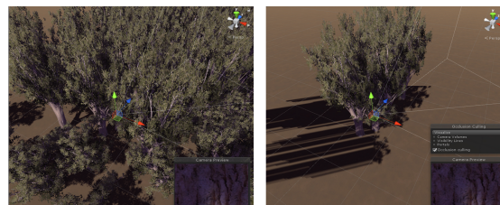
Figure 1. An example of occlusion culling. Left: No occlusion culling. Right: Full occlusion culling
