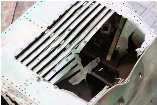
Figure 7. Major impact that tore the tanks roof apart [2]
